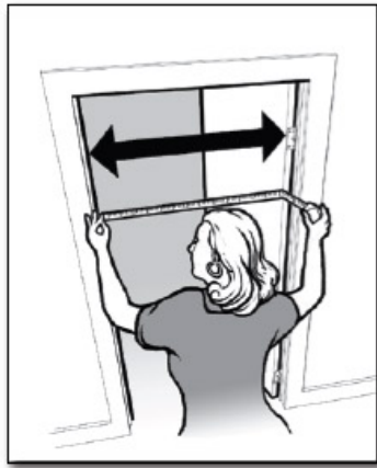
Measuring the clear opening from the face of the doorstop on the frame to the face of the open door
